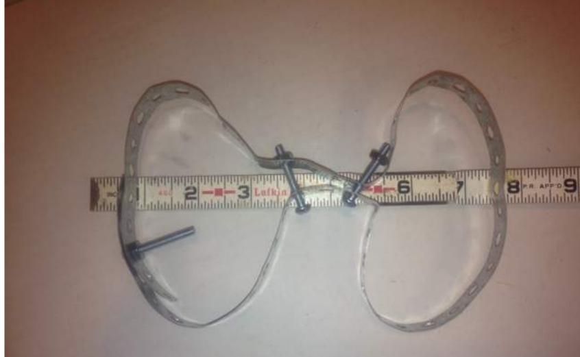
Cut a length of hanger strap about 28" long. Fasten the two ends together with a screw and nut. Then use two other screws and nuts to tighten the strap around the mounting pole.
